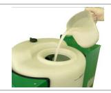
2.1.8 Feed water in quantities able to fill-up the EVA SYSTEM unit tank until the indicated "operating level" is reached.
