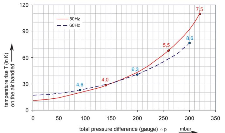
The performance curves are based on air at a temperature of 15 °C and an atmospheric pressure of 1013 mbar with a tolerance of +/- 10 %. The total pressure differences are valid for suction and ambient temperatures up to 25 °C. For other conditions please confer with us.
