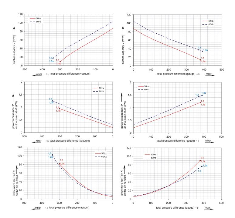
The performance curves are based on air at a temperature of 15  $^{\circ}$ C and an atmospheric pressure of 1013 mbar with a tolerance of +/- 10 %. The total pressure differences are valid for suction and ambient temperatures
